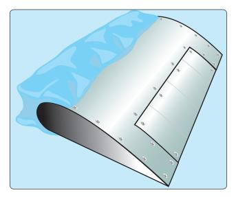
Figure 4-18. Clear ice buildup with horns.
