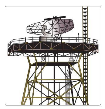
Figure 2-7. Combined radar and beacon antenna.
