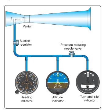
**Figure 5-27.** A venturi tube system that provides necessary vacuum to operate key instruments.
