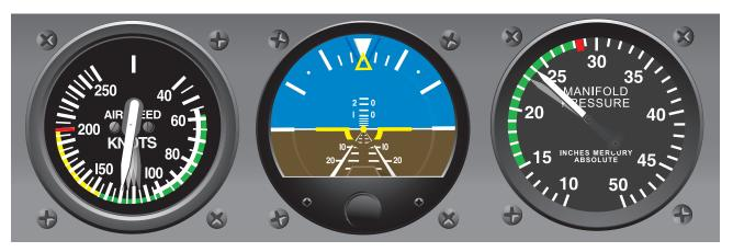
Figure 6-13. An increase in power—increasing airspeed accordingly in level flight.
