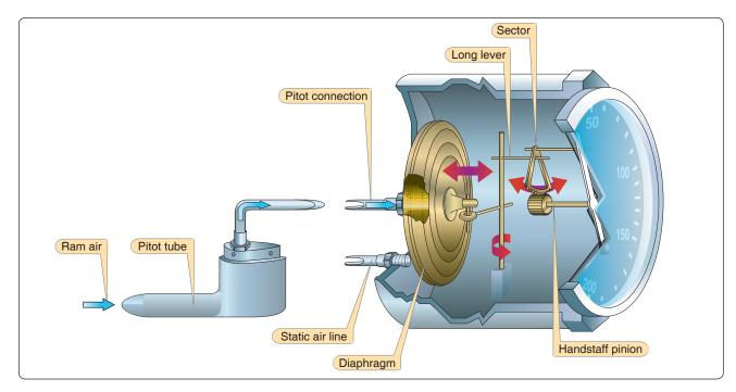
Figure 5-11. Mechanism of an ASI.
