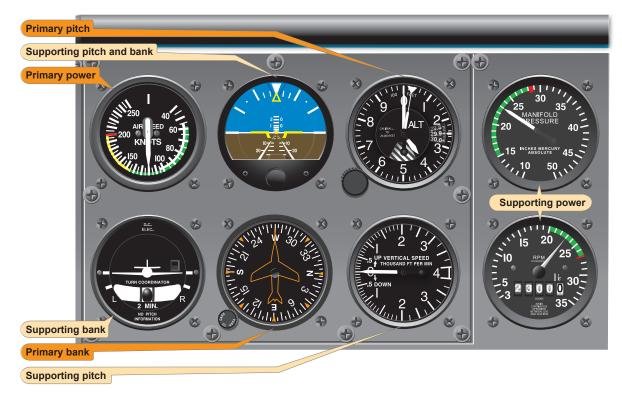
**Figure 7-22.** *Straight-and-level flight (normal cruising speed).*
