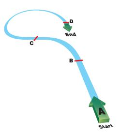
**Figure 7-43.** 80/260 procedure turn (entire pattern in level flight).
