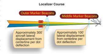
Figure 9-35. Localizer receiver indications and aircraft displacement.
