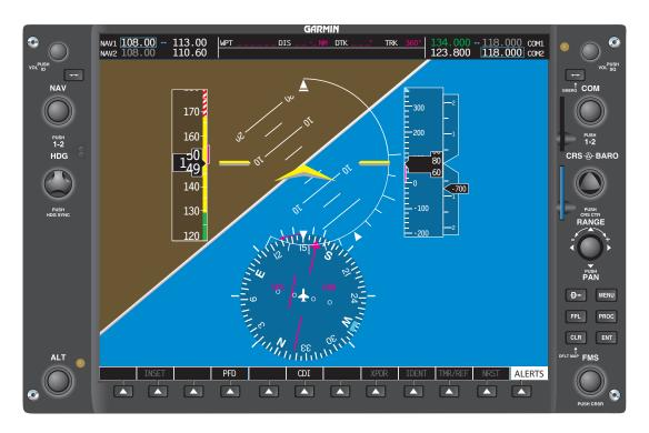
**Figure 7-71.** *Aircraft rolled past 60*°.
