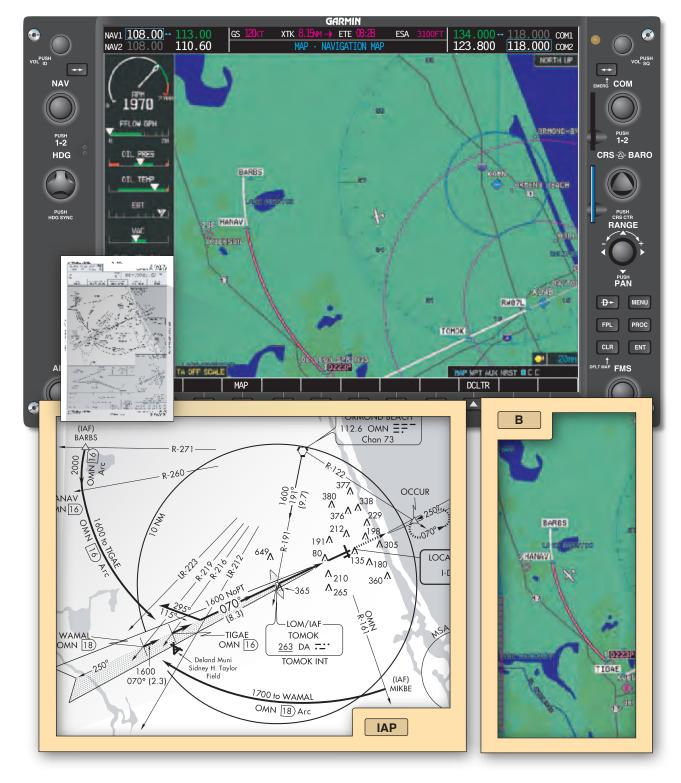
Figure 9-19. An aircraft is displayed heading southwest to intercept the localizer approach, using the 16 NM DME arc off of OMN.
