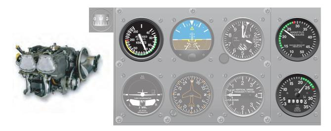
Figure 6-15. Power instruments.
