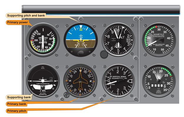
**Figure 7-30.** Constant airspeed descent, airspeed high—reduce power.
