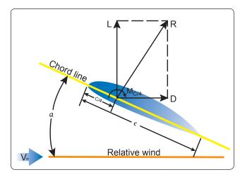
Figure 4-2. Angle of attack and relative wind.
