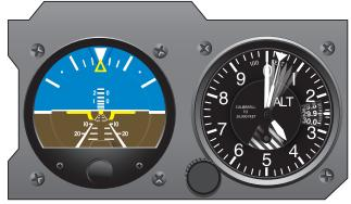
**Figure 6-7.** *Pitch correction using the altimeter.*
