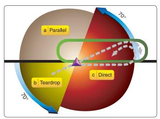
**Figure 10-6.** *Holding pattern entry procedures.*
