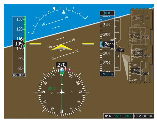
$\textbf{Figure 8-18.} \ \textit{PFD indications during a nose-low pitch attitude in a right turn.}$
