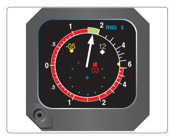
**Figure 5-58.** An example of a resolution advisory being provided to the pilot. In this case, the pilot is requested to climb, with 1,750 feet being the appropriate rate of ascent to avoid traffic conflict. This visual indication plus the audio warning provide the pilot with excellent traffic awareness that augments see-and-avoid practices.
