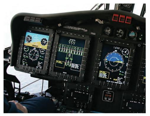
Figure 8-20. MFD display of aircraft systems.
