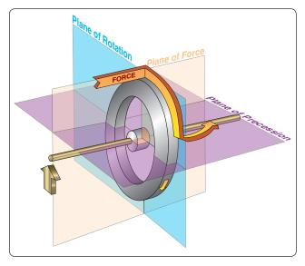
**Figure 5-32.** Precession causes a force applied to a spinning wheel to be felt 90° from the point of application in the direction of rotation.
