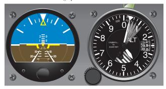
**Figure 7-8.** Pitch correction following altitude increase—lower nose to correct altitude error.
