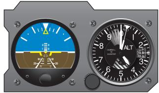
**Figure 6-6.** *Pitch correction using the attitude indicator.*
