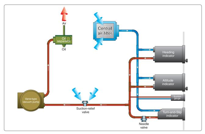
**Figure 5-28.** Single-engine instrument vacuum system using a steel-vane, wet-type vacuum pump.
