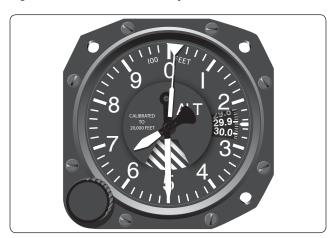
Figure 5-4. Three-pointer altimeter.
