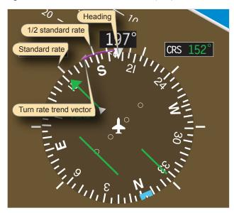
Figure 6-39. HSI indicator (enlargement).
