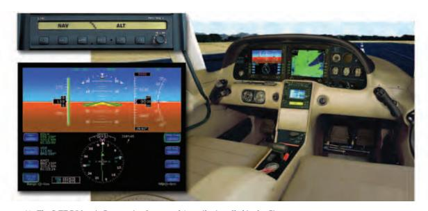
Figure 5-41. The S-TEC/Meggit Corporation Integrated Autopilot installed in the Cirrus.
