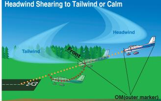
**Figure 10-17.** *Glideslope deviations due to wind shear encounter.*
