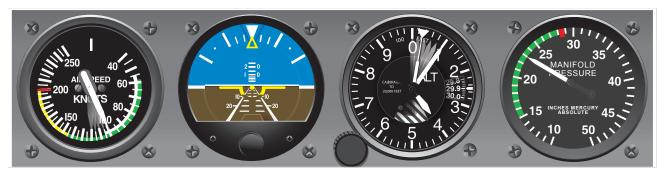
Figure 7-20. Airspeed low and altitude high—lower pitch.
