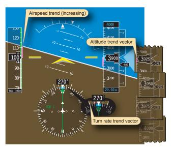
Figure 6-31. Supporting instruments.
