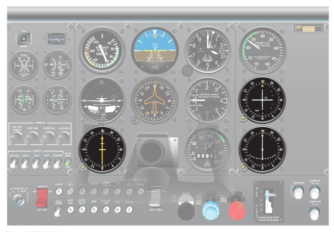
Figure 6-3. Navigation instruments.
