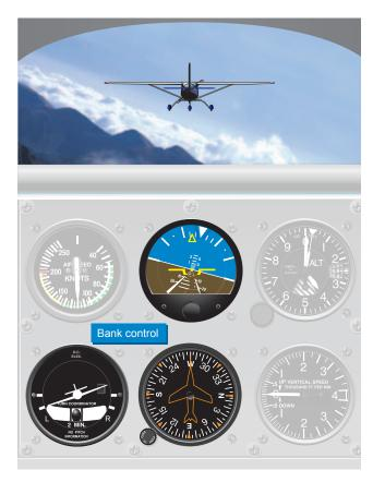
Figure 7-16. Instruments used for bank control.
