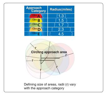
Figure 10-12. Circling approach area radii.
