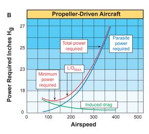
additional power is needed to maintain a slower airspeed. This region exists at speeds slower than the minimum drag point (L/ $D_{MAX}$ ) on the thrust required curve, *Figure 4-9*) and is primarily due to induced drag. *Figure 4-10* shows how one power setting can yield two speeds, points 1 and 2. This is because at point 1 there is high induced drag and low parasite drag, while at point 2 there is high parasite drag and low induced drag.
