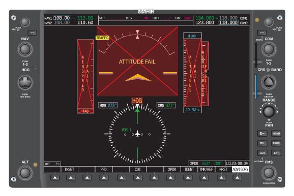
Figure 7-74. AHRS ADC failure.
