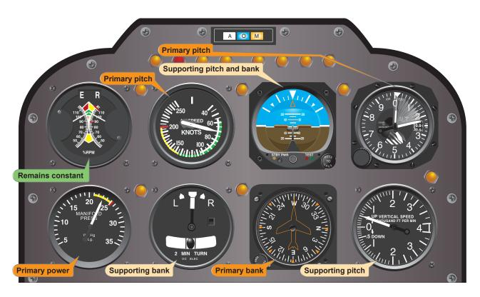
Figure 8-11. Flight instrument indications during climb entry for a constant-airspeed climb.
