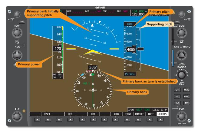
**Figure 7-67.** *Standard rate turn—constant airspeed.*
