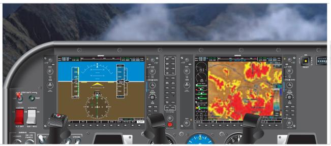
Figure 7-48. Pitch attitude decreasing and airspeed increasing—indicates need to increase pitch.
