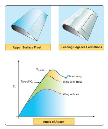
Figure 4-21. Effect of ice and frost on lift.
