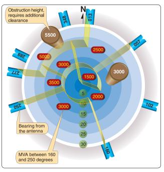
Figure 2-8. Minimum vectoring altitude (MVA) chart.
