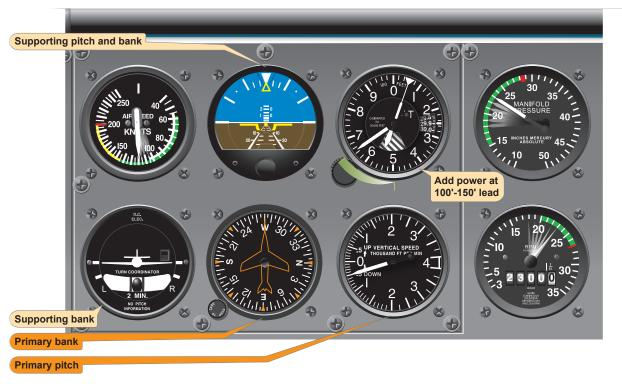
Figure 7-31. Level off airspeed higher than descent airspeed.
