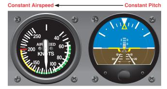
Figure 7-13. Constant power plus constant pitch equals constant speed.
