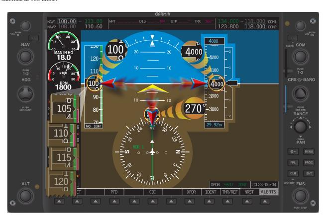
Figure 7-61. Insufficient cross-check. The problem is power and not nose-high. In this case, the pilot decreased pitch inappropriately.
