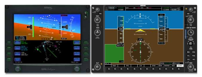
Figure 5-45. Two primary flight displays (Avidyne on the left and Garmin on the right).
