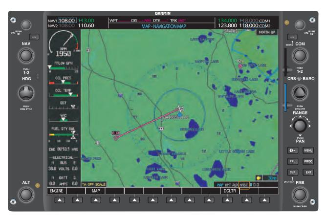
**Figure 11-13.** *The MFD is another means of viewing the nearest airports.*
