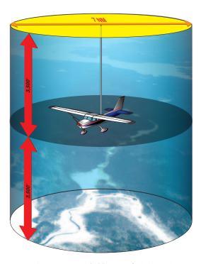
**Figure 5-52.** Coverage provided by a traffic information system.
