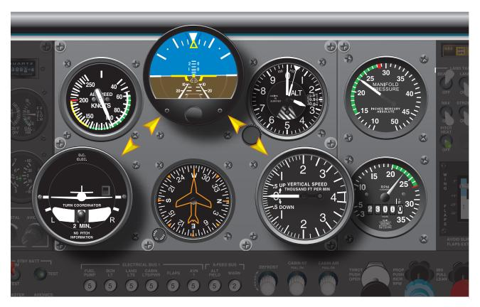
Figure 6-18. Inverted-V cross-check.
