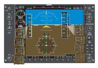
**Figure 7-55.** An aircraft decreasing in airspeed while gaining altitude. In this case, the pilot has decreased pitch.
