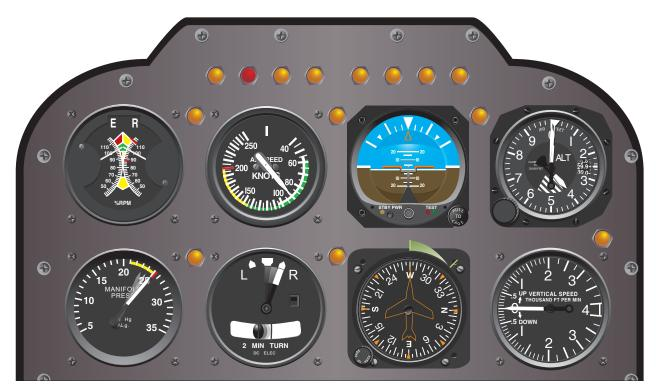
Figure 8-7. Flight instrument indications in straight-and-level flight with power increasing.
