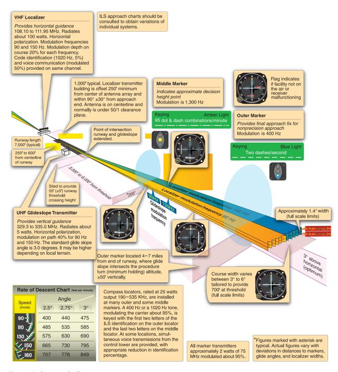
Figure 9-33. Instrument landing systems.
