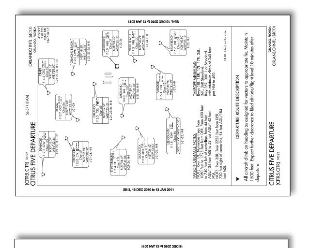
$\overline{f V}$  Take-off minimums and (obstacle) departure procedures  $\overline{f V}$
