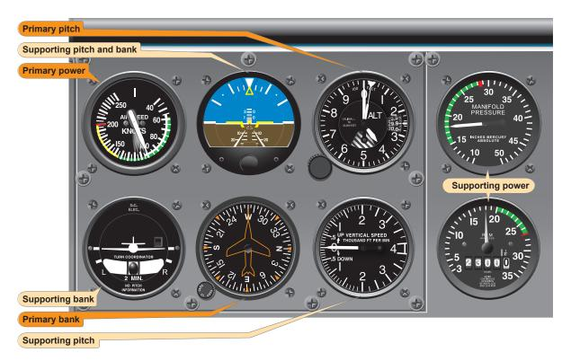
Figure 7-24. Straight-and-level flight (reduced airspeed stabilized).
