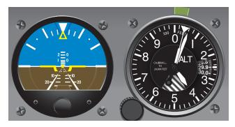
Figure 7-9. Altitude error, less than 100 feet.
