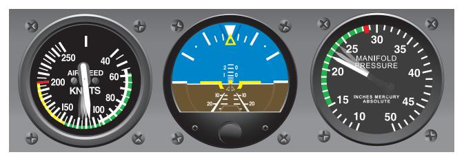
**Figure 6-14.** Pitch control and power adjustment required to bring aircraft to level flight.
