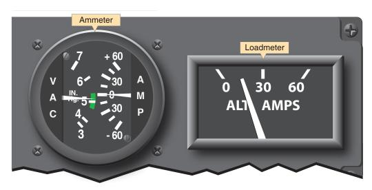
Figure 11-4. Ammeter (left) and loadmeter (right).
