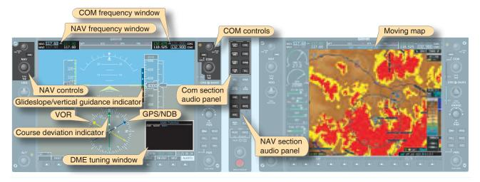
Figure 6-27. Navigation instruments.
