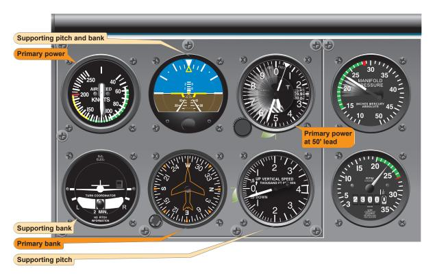
Figure 7-32. Level off at descent airspeed.
