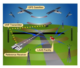
**Figure 9-32.** The LAAS system working with GPS satellites, reference receivers and radio transmitters which are located on or in the vicinity of the airport.
