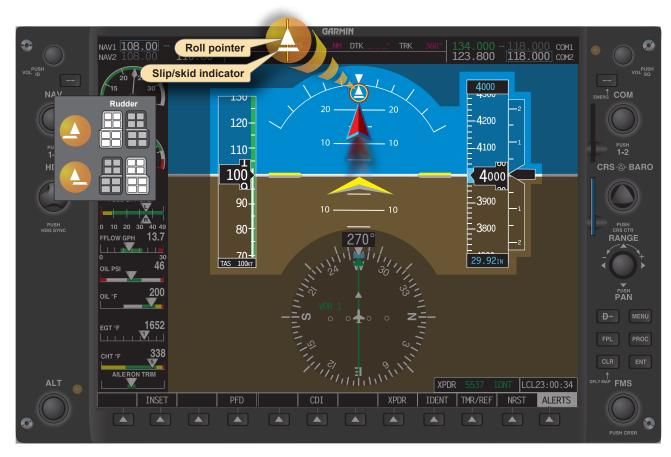
**Figure 6-34.** *Roll pointer and slip/skid indicator.*
