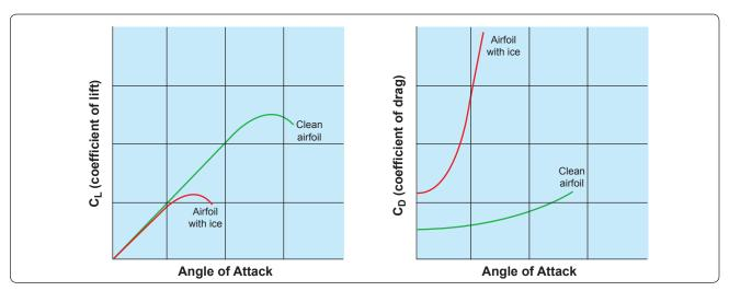
Figure 4-20. Aerodynamic effects of icing.
