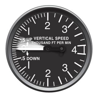
Figure 6-8. Vertical speed indicator.
