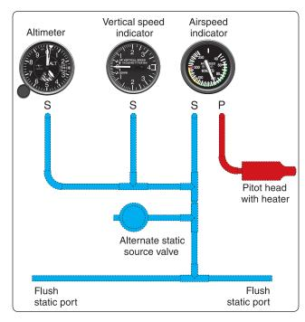
Figure 5-2. A typical pitot-static system.
