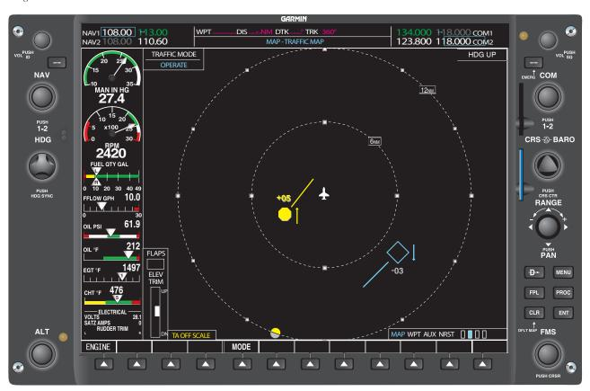
**Figure 11-18.** A typical display on aircraft MFD when using TIS.
