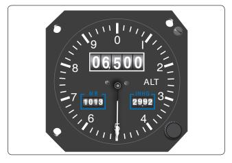
Figure 5-5. Drum-type altimeter.
