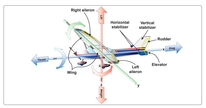
**Figure 4-3.** *The four forces and three axes of rotation.*
