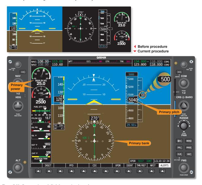
Figure 7-63. Constant airspeed climb from cruise airspeed.
