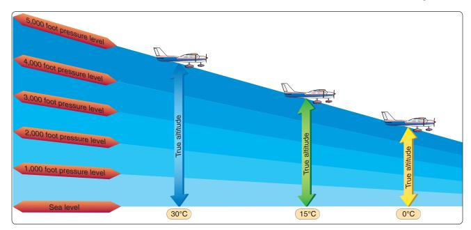
Figure 5-6. The loss of altitude experienced when flying into an area where the air is colder (more dense) than standard.
