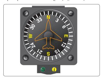
Figure 5-22. Vertical card magnetic compass.
