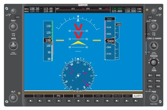
Figure 7-69. Unusual attitude recovery protection. Note the brown horizon line is visible at the bottom.
