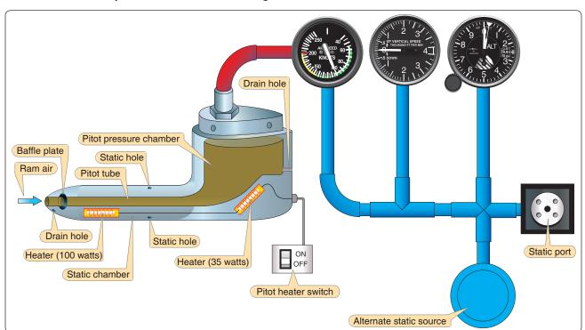
**Figure 5-1.** A typical electrically heated pitot-static head.
