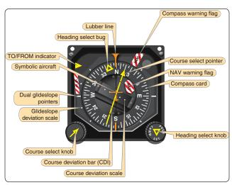
Figure 5-38. Horizontal situation indicator (HSI).
