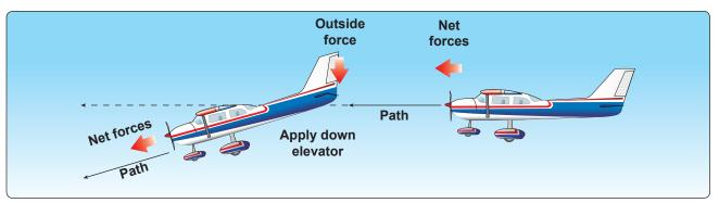
Figure 4-4. Newton's First Law of Motion: the Law of Inertia.
