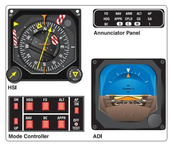
Figure 5-40. Components of a typical FDS.
