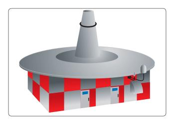
Figure 9-11. VOR transmitter (ground station).
