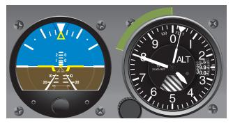
Figure 7-11. Altitude error, greater than 100 feet.
