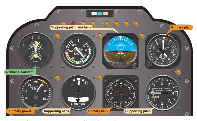
$\textbf{Figure 8-9.} \ \textit{Flight instrument indications in straight-and-level flight at normal cruise speed.}$
