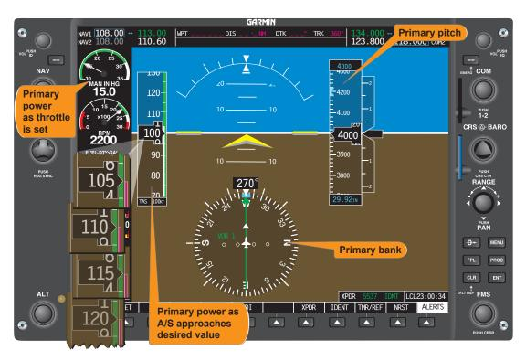
**Figure 7-58.** *Straight-and-level flight (airspeed decreasing).*
