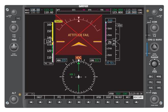
Figure 7-73. AHRS unit failed.
