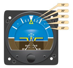
**Figure 5-30.** The dial of this attitude indicator has reference lines to show pitch and roll.
