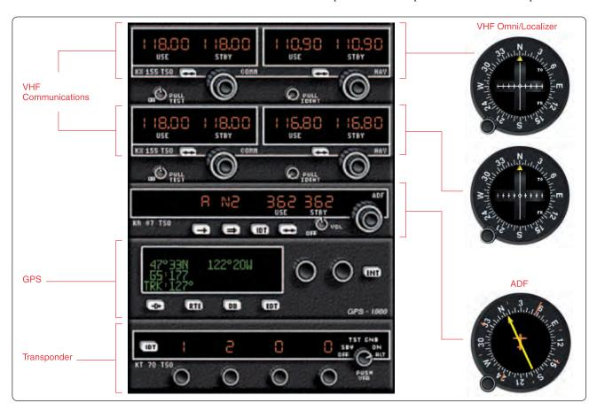
Figure 2-1. Typical navigation/communication installation.
