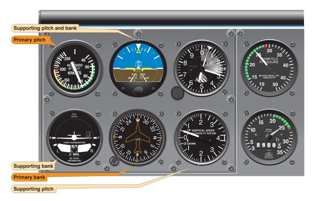
Figure 7-26. Stabilized climb at constant airspeed.
