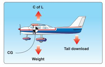
**Figure 4-22.** *Downward force on the tailplane.*
