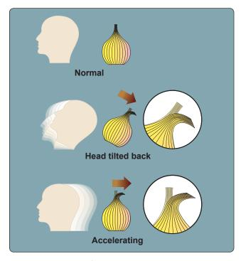
Figure 3-6. Linear acceleration.
