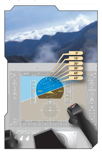
Figure 6-29. Bank indicator index lines.
