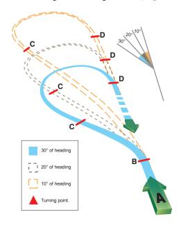
**Figure 7-44.** Teardrop pattern (entire pattern in level flight).
