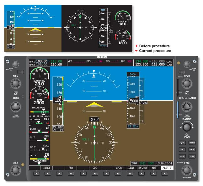
**Figure 7-66.** The top image illustrates a reduction of power and descending at 500 fpm to an altitude of 5,000 feet. The bottom image illustrates an increase in power and the initiation of leveling off.
