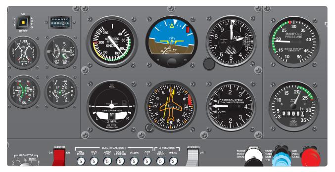
Figure 11-8. Vacuum failure.
