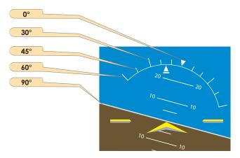
**Figure 7-53.** *Attitude indicator showing a 15° left bank.*
