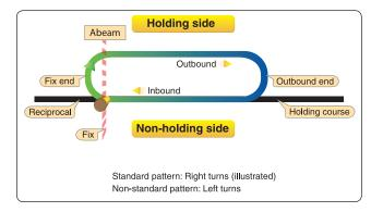
Figure 10-4. Standard holding pattern—no wind.
