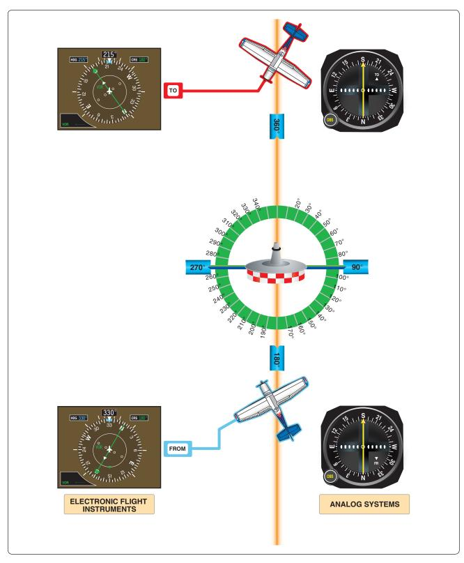
$\textbf{Figure 9-15.} \ CDI \ interpretation. \ The \ CDI \ as \ typically found \ on \ analog \ systems \ (right) \ and \ as found \ on \ electronic \ flight \ instruments \ (left).$
