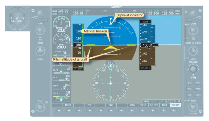
Figure 6-30. Pitch of the aircraft.
