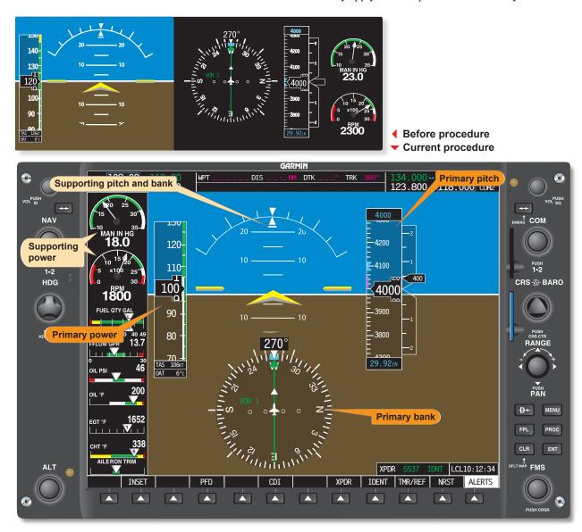
Figure 7-64. Constant airspeed climb from established airspeed.
