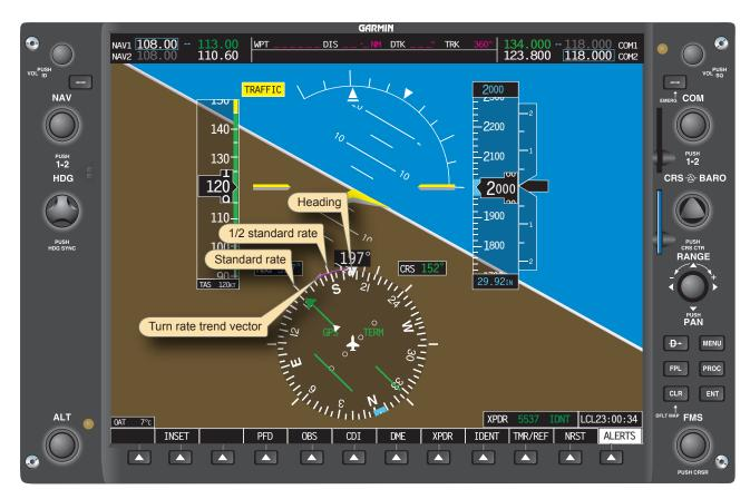
Figure 6-38. Horizontal situation indicator (HSI) trend indicator elongates proportionally with the rate of turn.
