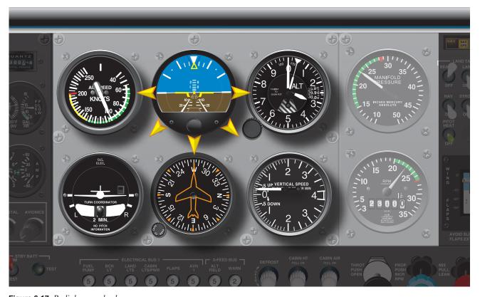
Figure 6-17. Radial cross-check.
