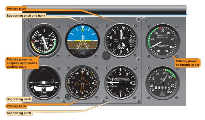
Figure 7-23. Straight-and-level flight (airspeed decreasing).
