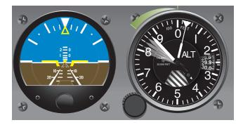
**Figure 7-12.** Pitch correction, greater than 100 feet—one bar correction initially.
