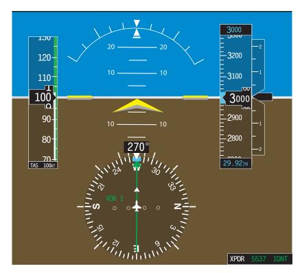
Figure 8-17. PFD indications during straight-and-level flight.
