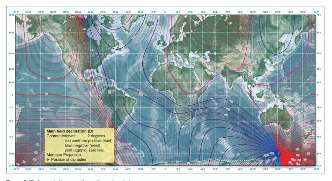
Figure 5-17. Isogonic lines are lines of equal variation.
