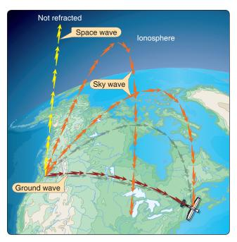
**Figure 9-1.** *Ground, space, and sky wave propogation.*
