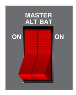
Figure 11-5. Double rocker switch seen on many aircraft.
