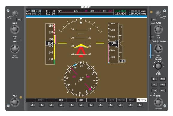
Figure 7-70. Horizon line starts moving upward at 27°. Note that the blue sky remains visible at 17° nose-down.
