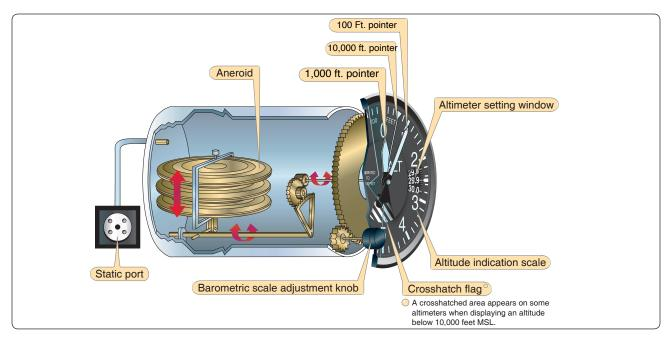
Figure 5-3. Sensitive altimeter components.
