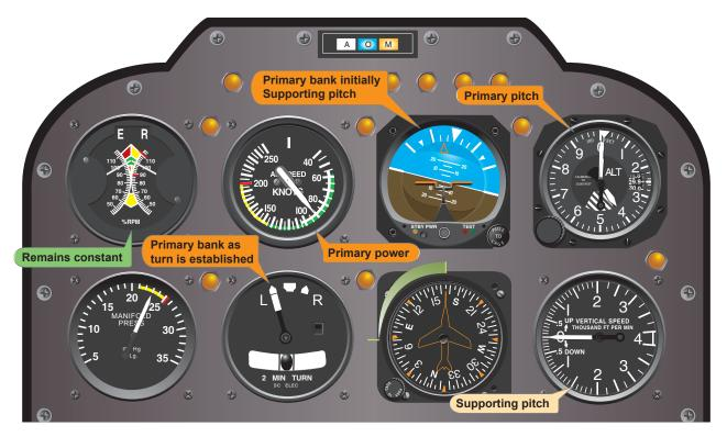
Figure 8-14. Flight instrument indications in a standard-rate turn to the left.
