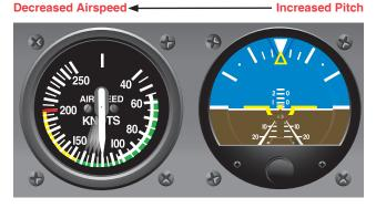
**Figure 7-15.** Constant power plus increased pitch equals decreased airspeed.
