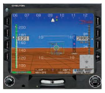
**Figure 5-46.** The benefits of realistic visualization imagery, as illustrated by Synthetic Vision manufactured by Chelton Flight Systems. The system provides the pilot a realistic, real-time, three-dimensional depiction of the aircraft and its relation to terrain around it.
