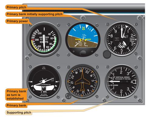
Figure 7-33. Standard rate turn, constant airspeed.
