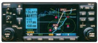
Figure 2-4. Combination GPS-com unit.
