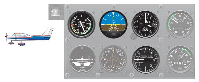
Figure 6-4. Pitch instruments.
