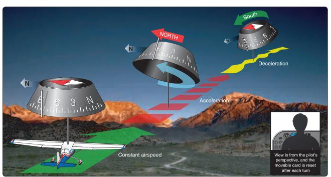
**Figure 5-21.** *The effects of acceleration error.*
