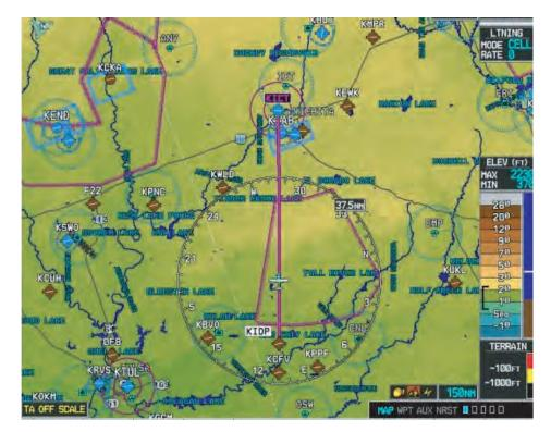
Figure 8-19. MFD display of a moving map.
