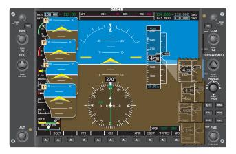
**Figure 7-50.** *Pitch indications for various attitudes* ( $1^{\circ}$  *through*  $5^{\circ}$ ).
