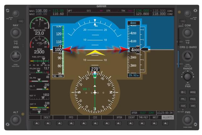
Figure 7-62. The pilot has fixated on pitch and altitude, leaving bank indications unattended. Note the trend line to the left.
