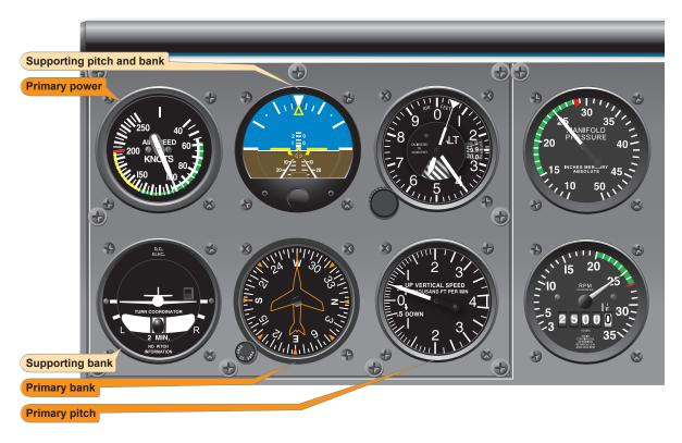
Figure 7-27. Stabilized climb at constant rate.
