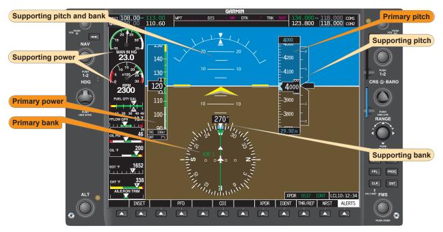
Figure 7-57. Straight-and-level flight (normal cruising speed).
