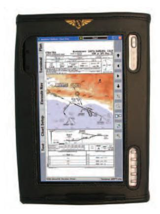
**Figure 1-7.** Example of an electronic flight bag.
