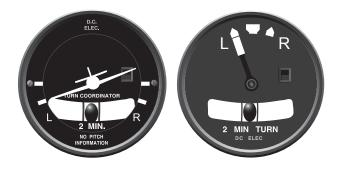
Figure 6-12. Turn coordinator and turn-and-slip indicator.
