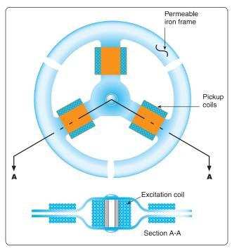
**Figure 5-23.** The soft iron frame of the flux valve accepts the flux from the Earth's magnetic field each time the current in the center coil reverses. This flux causes current to flow in the three pickup coils.
