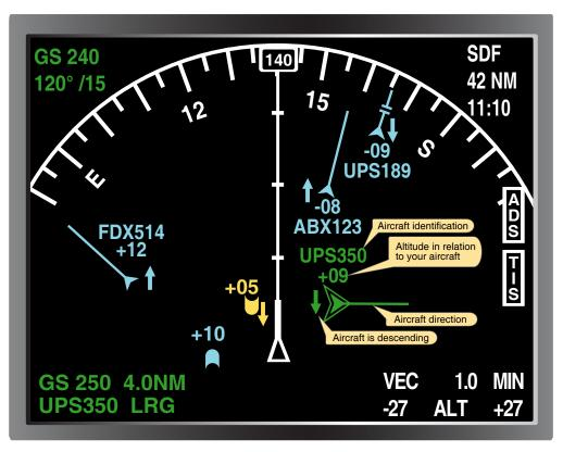
Figure 5-49. An aircraft equipped with ADS will receive identification, altitude in hundreds of feet (above or below using + or-), direction of the traffic, and aircraft descent or climb using an up or down arrow. The yellow target is an illustration of how a non-ADS equipped aircraft would appear on an ADS-equipped aircraft's display.
