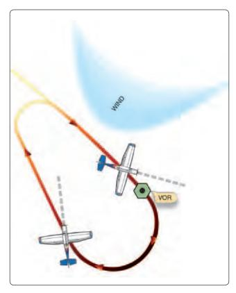
**Figure 10-5**. *Drift correction in holding pattern.*
