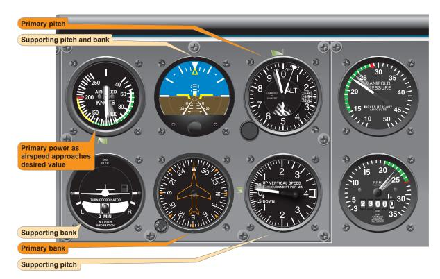
Figure 7-29. Level off at cruising speed.
