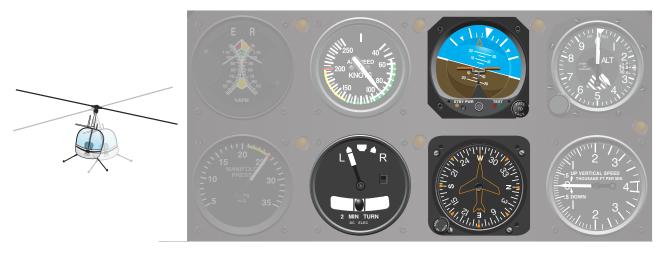
Figure 8-4. The flight instruments used for bank control are the attitude, heading, and turn indicators.
