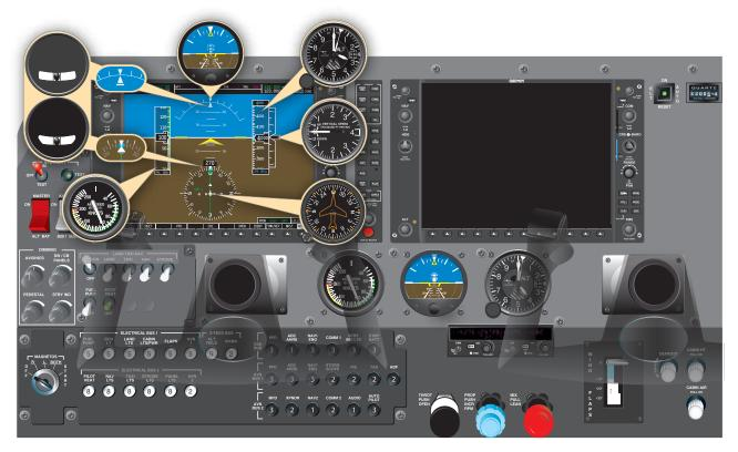
Figure 6-21. Primary flight display (PFD) and analog counterparts.
