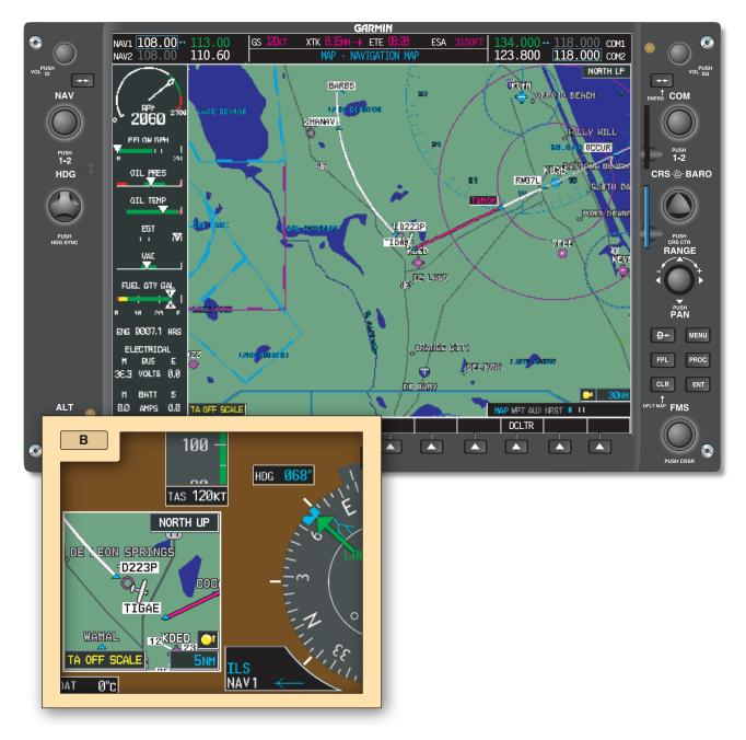
**Figure 9-20.** The same aircraft illustrated in Figure 9-19 shown on the OMN radial near TIGAE intersection turning inbound for the localizer.
