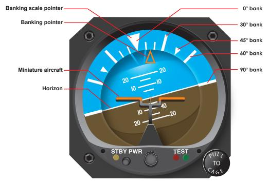
**Figure 8-5.** The banking scale at the top of the attitude indicator indicates varying degrees of bank. In this example, the helicopter is banked approximately 15° to the right.
