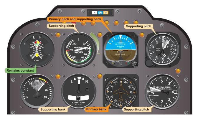
**Figure 8-16.** Flight instrument indications during an instrument takeoff.
