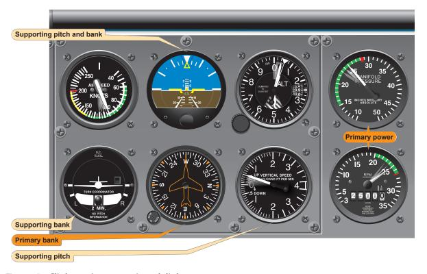
Figure 7-25. Climb entry for constant airspeed climb.
