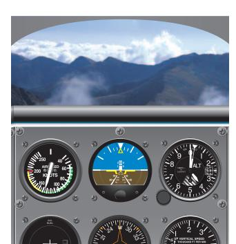
**Figure 7-2.** Pitch attitude and airspeed in level flight, fast cruise speed.
