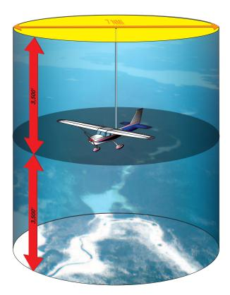
pilot. Systems such as TIS provide a visual representation of nearby traffic and displays a symbol on the moving map display with relative information about altitude, vertical trends, and direction of flight. [Figure 11-18]
