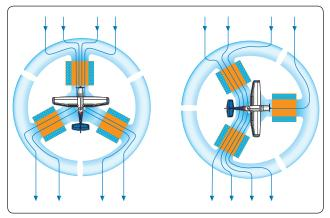
**Figure 5-24.** *The current in each of the three pickup coils changes with the heading of the aircraft.*
