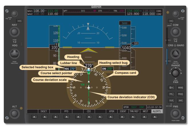
**Figure 9-14.** An HSI display as seen on the pilot's primary flight display (PFD) on an electronic flight instrument. Note that only attributes related to the HSI are labeled.
