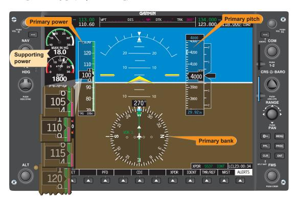
$\textbf{Figure 7-59.} \ \textit{Straight-and-level flight (reduced airspeed stabilized)}.$
