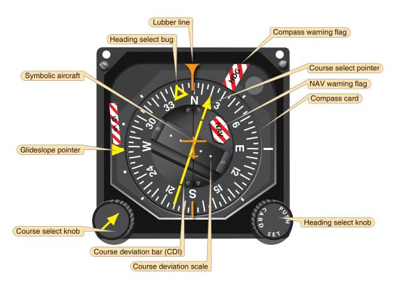
Figure 9-13. A typical horizontal situation indicator (HSI).
