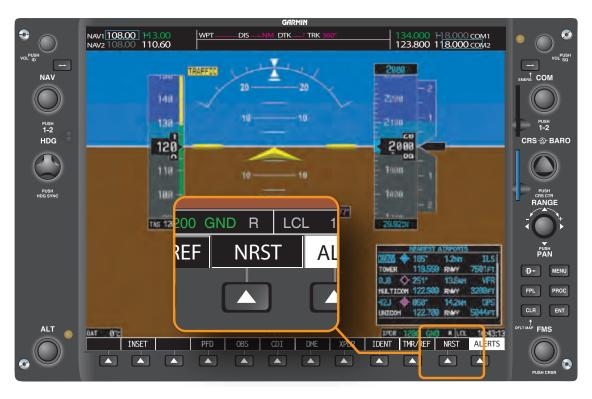
**Figure 11-9.** The default soft key menu that is displayed on the PFD contains a "NRST" (Nearest Airport) soft key. Pressing this soft key opens a text box that displays the nearest 25 airports.
