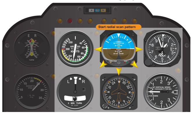
**Figure 8-1.** A radial scan pattern of the flight instruments enables the helicopter pilot to fully comprehend the condition and direction of the helicopter.
