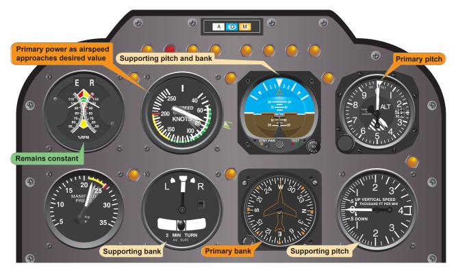
Figure 8-10. Flight instrument indications in straight-and-level flight with airspeed decreasing.
