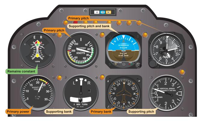
**Figure 8-12.** Flight instrument indications in a stabilized constant-airspeed climb.
