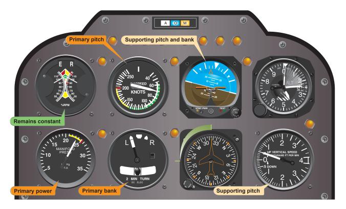
Figure 8-15. Flight instrument indications for a stabilized left climbing turn at a constant airspeed.
