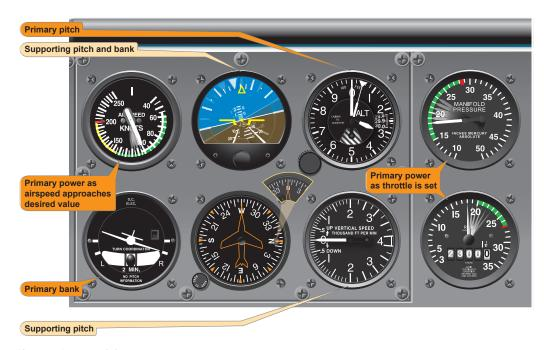
Figure 7-38. Change of airspeed during turn.
