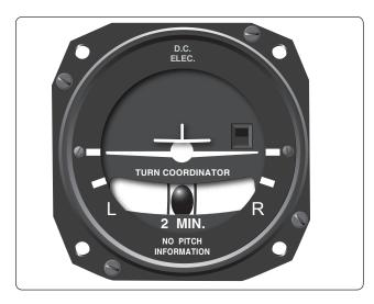
**Figure 5-35.** A turn coordinator senses rotation about both roll and yaw axes.
