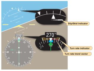
Figure 7-54. Slip/skid and turn rate indicator.
