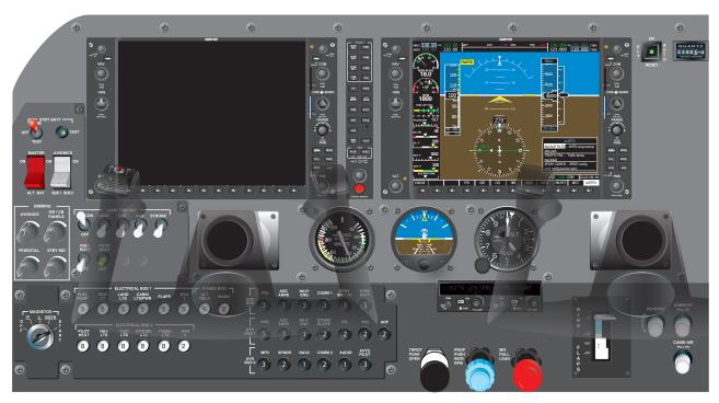
Figure 6-23. Reversionary displays.
