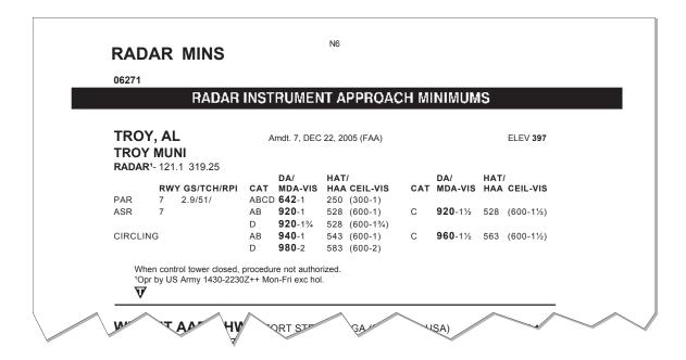
Figure 10-10. Radar instrument approach minimums for Troy, Alabama.
